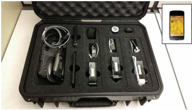
Fig. 1. The Canadian snipers NABK ballistic computer kit with the various sensor connectors and power pack.
