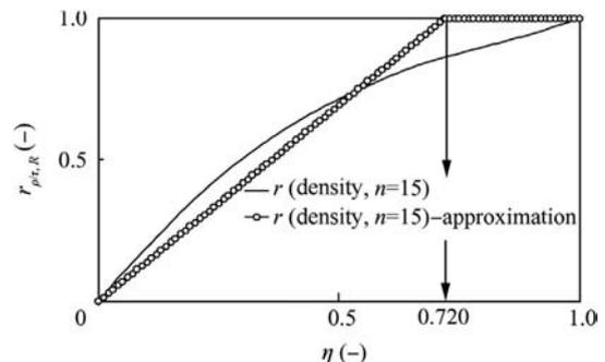
Fig. 4. WFF for the air density  $\rho$  (concave shape)  $r_{p/r,R}(\eta)$ ,  $Y_s = 18\,000$  m,  $S = 0.640$ ,  $K_{CR} = 0.720$ ,  $Y_R = \Delta h_{R2} = 13\,000$  m [1,6].
