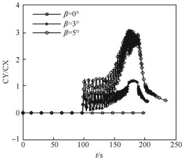
Fig. 9. Curves of lift-drag ratio with deflection angle  $\beta = 0^\circ, 3^\circ$  and  $5^\circ$ .
