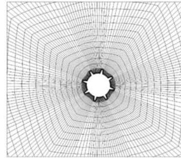
(b) View of the missile-tail mesh in the cross section of  $x$  axis
