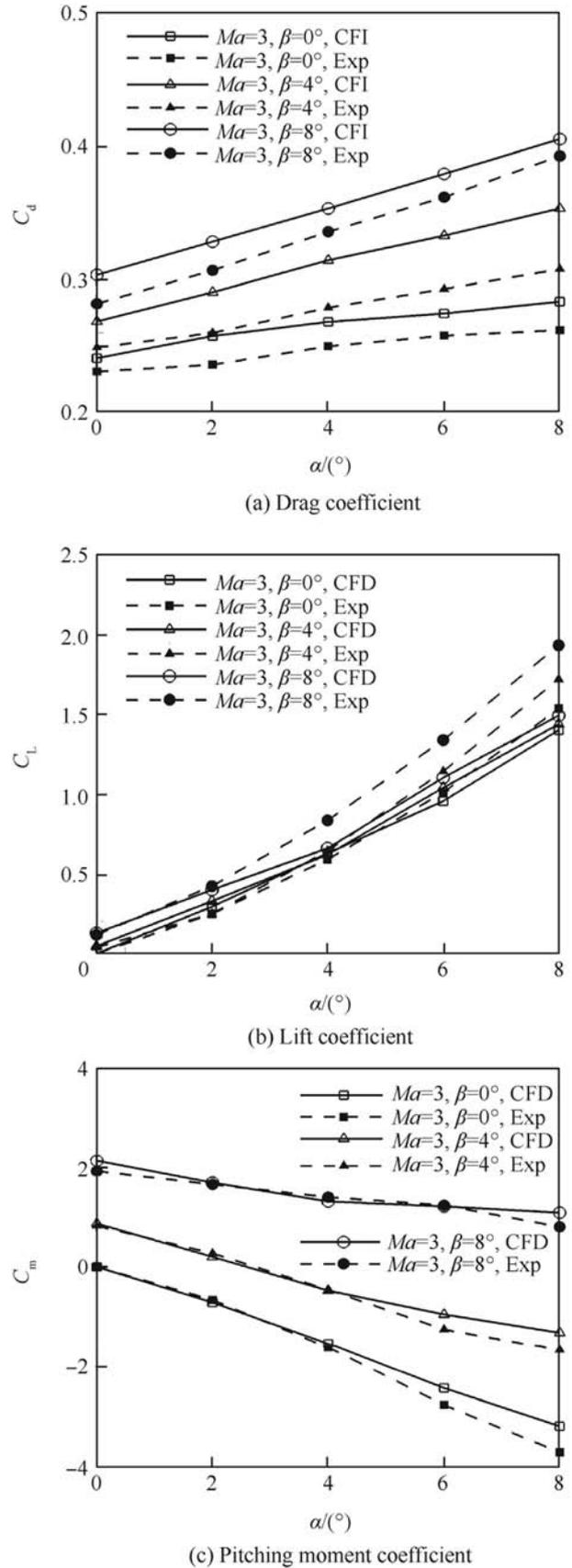
Fig. 4. Comparison of experimental aerodynamic coefficients [2] with our numerical results under  $Ma = 3$  and attack of angles.
