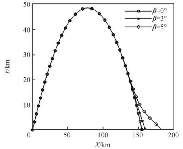
Fig. 6. Trajectory of deflected missile with different deflection angle.
