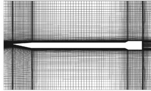
(a) View of the missile-tail mesh in the longitudinal direction
