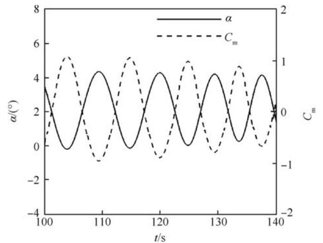
Fig. 7. Time histories of both of the angle of attack and pitching moment coefficient.
