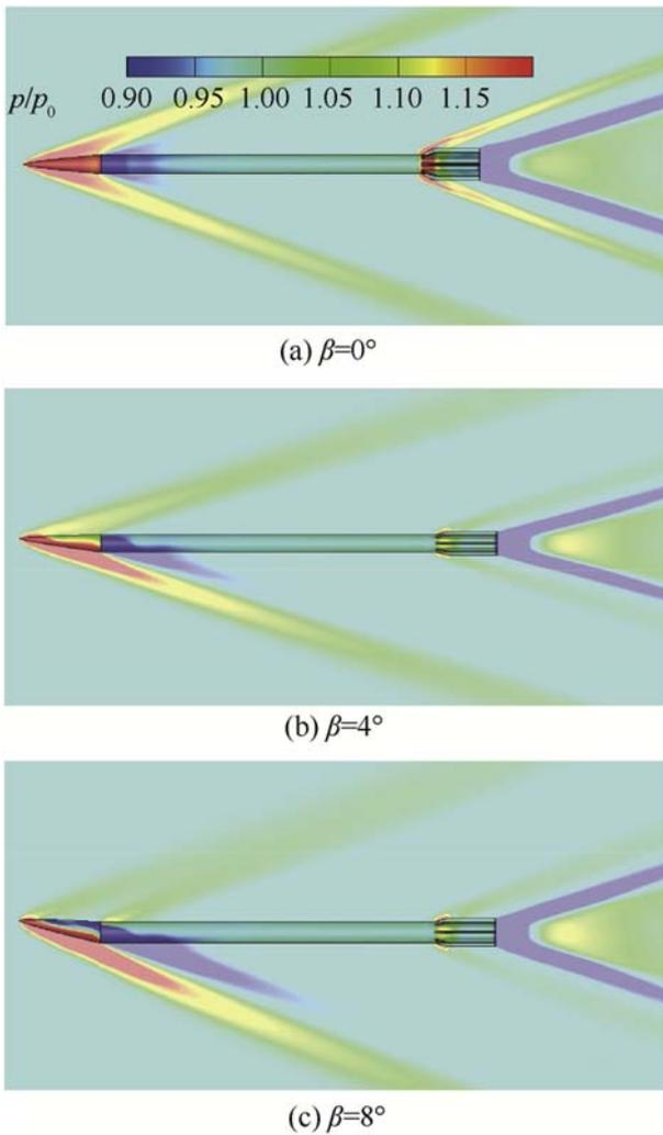
Fig. 3. Pressure contours of a deflectable missiles at  $Ma = 3.0$ ,  $\alpha = 0^\circ$  and different deflection angles  $\beta = 0^\circ$ ,  $4^\circ$  and  $8^\circ$ .
