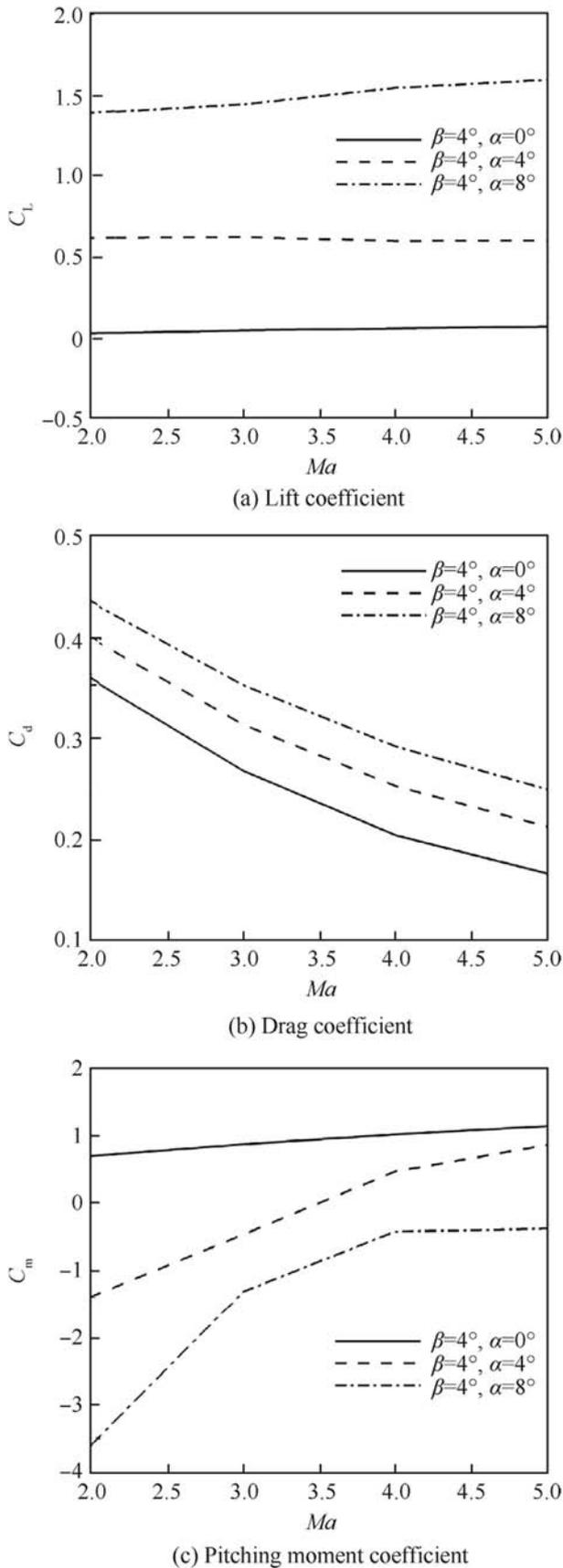
Fig. 5. Aerodynamic coefficients of the missile with  $\beta = 4^\circ$  and different mach numbers.
