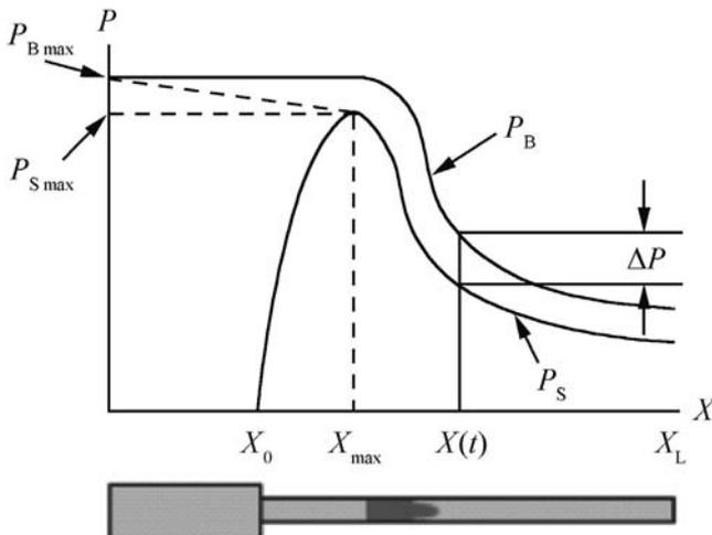
Fig. 3. Typical barrel internal ballistic. Pressure-distance graph [5].
