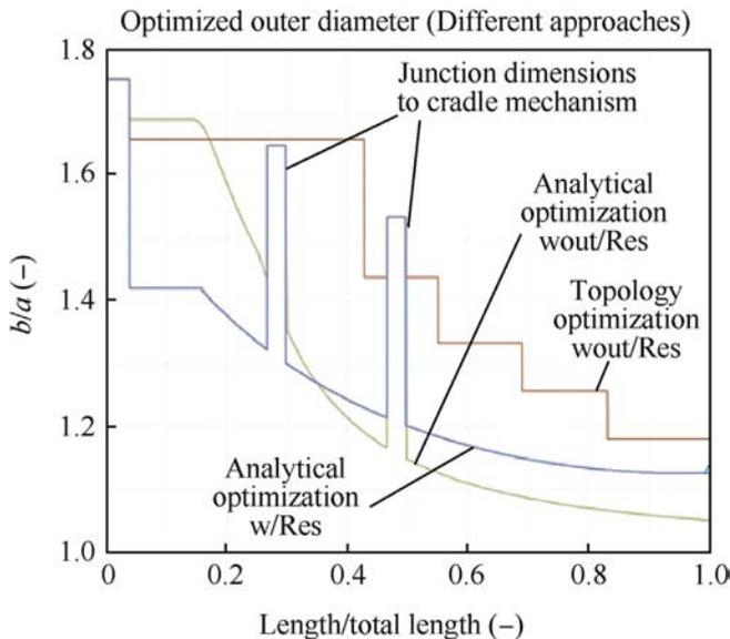
Fig. 12. Comparison of analytically optimized and topology optimized models with a safety coefficient of 1.0.
