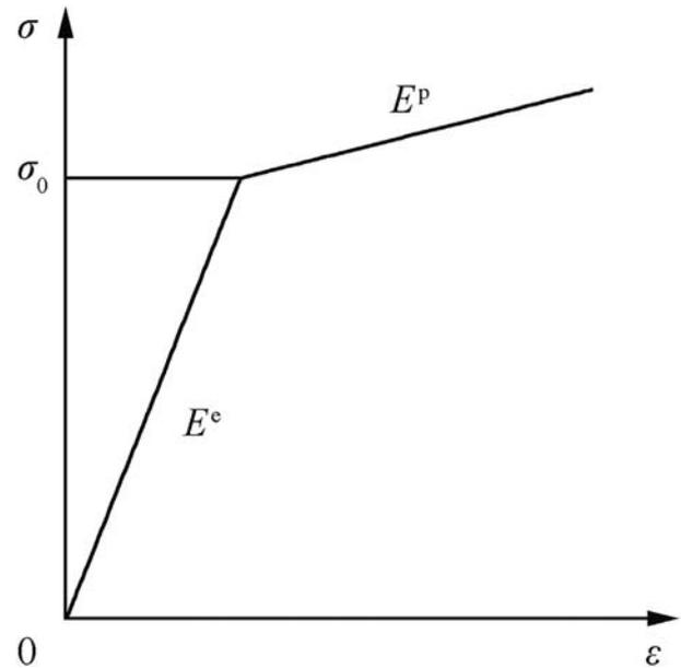
Fig. 1. Elastic-linear plastic material model.
