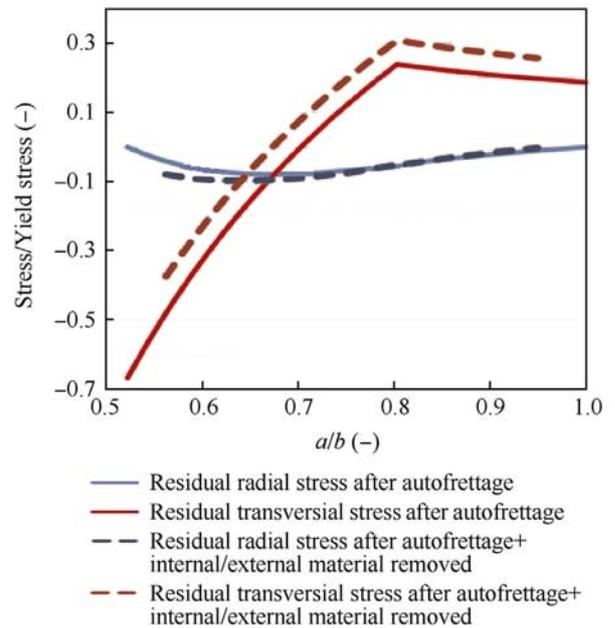
Fig. 7. Comparison of residual stresses after autofrettage and stresses in the case of internal and external material removal after autofrettage.
