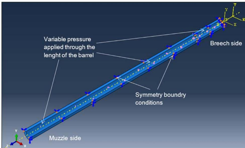
Fig. 6. Topology Optimization model boundary and loading conditions.
