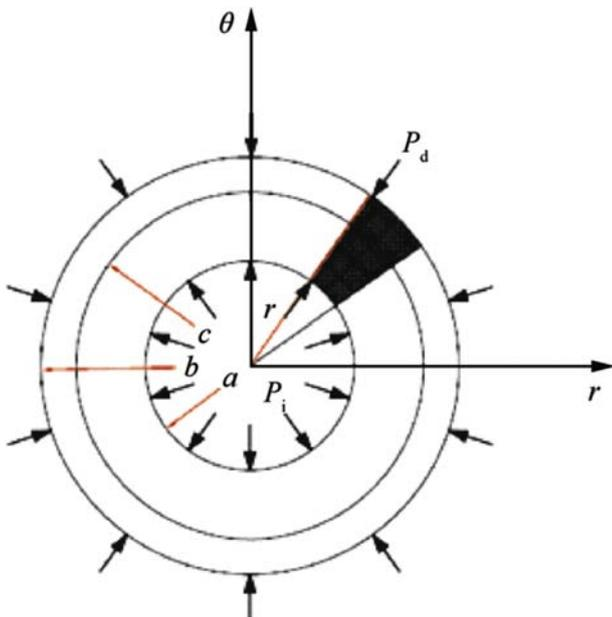
Fig. 2. Common loading and radii representation of a thick wall cylinder.
