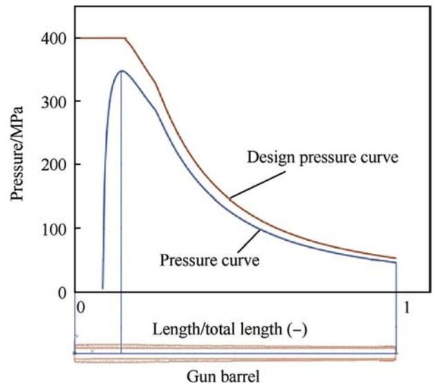
Fig. 4. Internal ballistic pressure distribution curves and corresponding points on the barrel.
