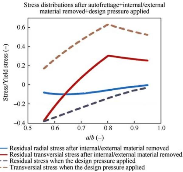
Fig. 8. Stress distribution for autofrettaged + material removed and service pressure applied.
