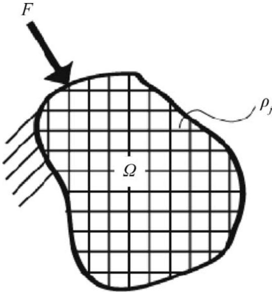
Fig. 5. Abstract model of design space showing load and boundary conditions [8].
