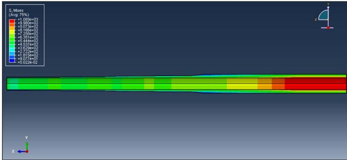
Fig. 10. The weight optimized half symmetrical model.
