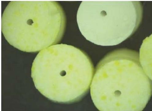
Fig. 14. Blotchy coat on Surface of inert CAB substrate.
