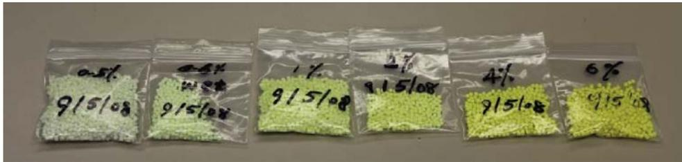
Fig. 13. UV Curable coatings with varying concentration (0.5%, 0.6%, 1%, 2%,4%,6% on inert CAB substrate.
