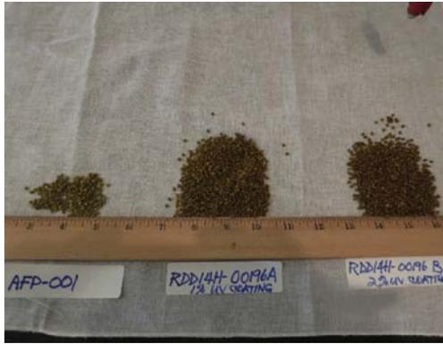
**Fig. 16.** AFP-001 AND LED UV Surface Coated Energetic Propellant AFP-001 (Uncoated Grain Dimensions: Length = 0.096 inch, Diameter = 0.083 inch, Perf Diameter = 0.006 inch, Average Web Size = 0.038 inch).
