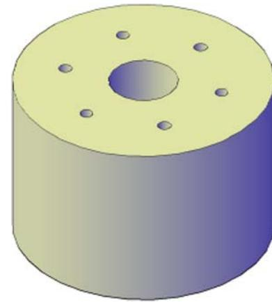
Fig. 6. Schematic diagram of molded 7-perf propellant.
