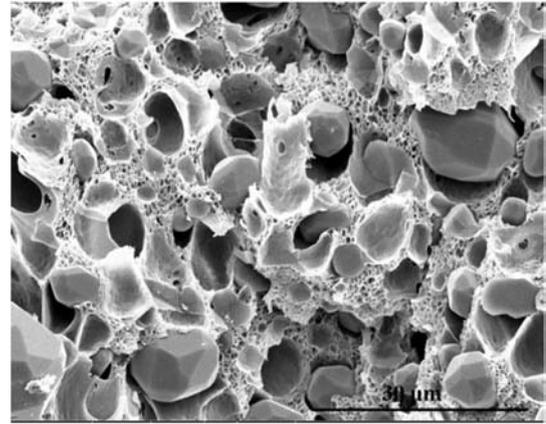
Fig. 2. SEM micrograph of foamed combustible materials.
