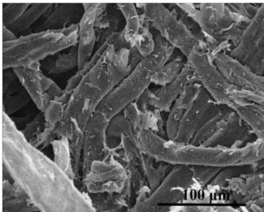
Fig. 1. SEM micrograph of felted combustible material.
