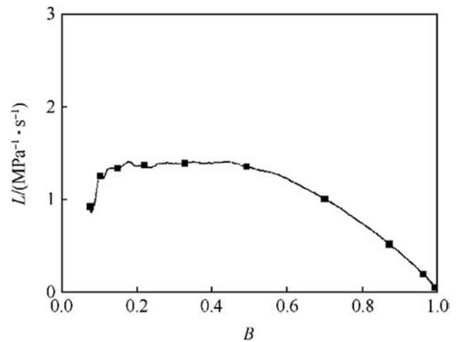
Fig. 7. *L-B* curve of consolidated propellant.
