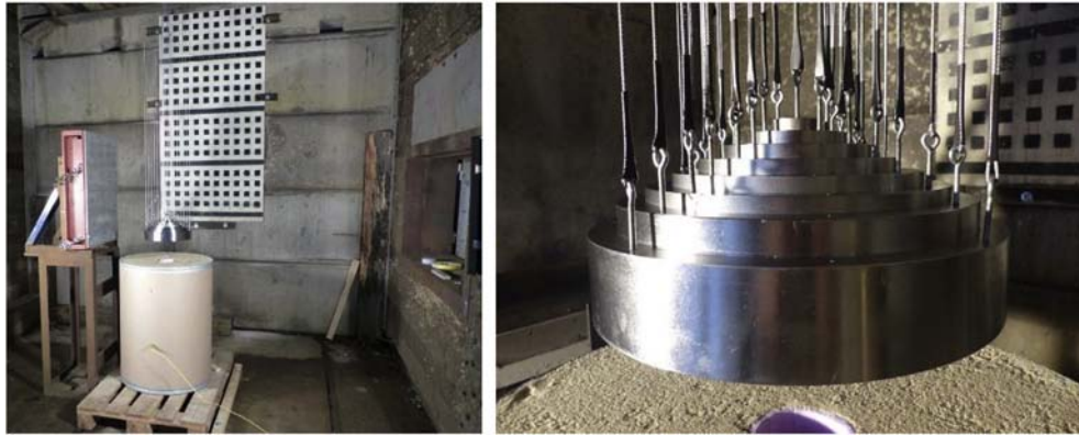
Fig. 1. Measurement setup with concentric rings suspended at wire cables (left), screw connection of the wire cables at the rings (right).
