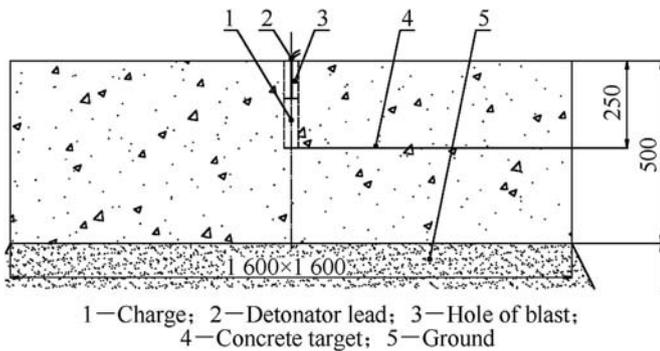
**Fig. 3.** Layout of explosive charge in the slab.
