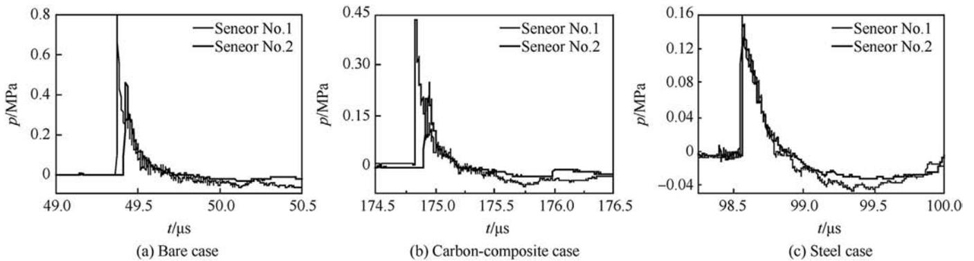
Fig. 5. The testing overpressure-time curves of the three charges.
