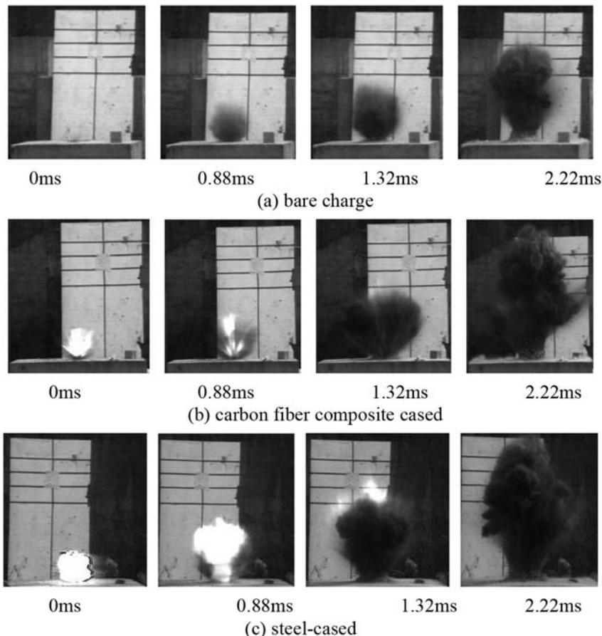
Fig. 8. High speed photographs of blasting in concrete for the three charges.
