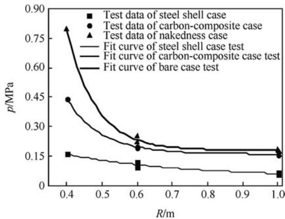
Fig. 6. Overpressure fitting curves of the three charges [5].
