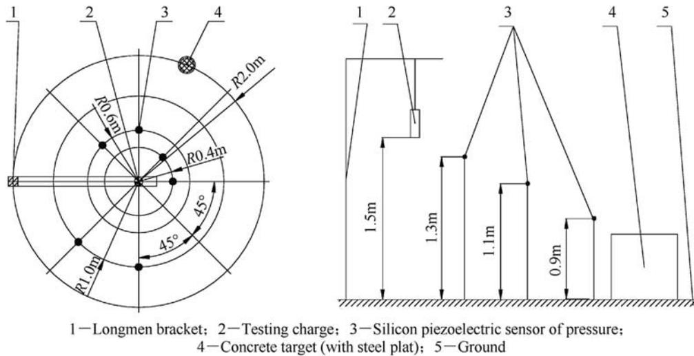
**Fig. 2.** Schematic diagram of air blast experimental layout.
