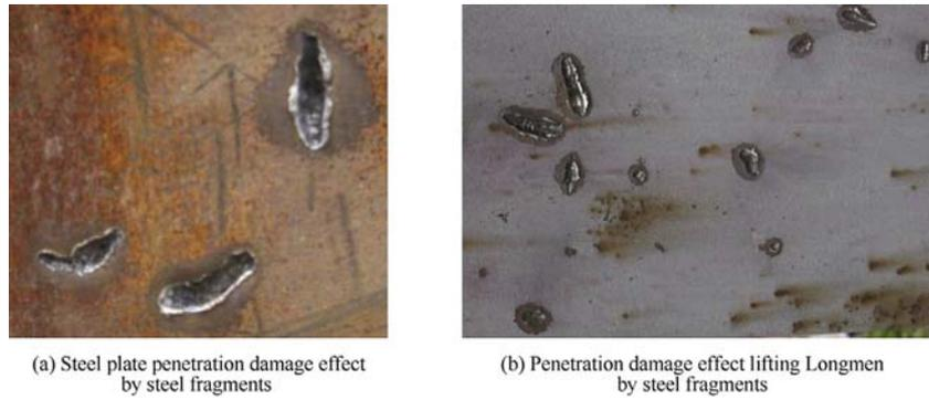
Fig. 4. Damage of steel fragments from the air blast.
