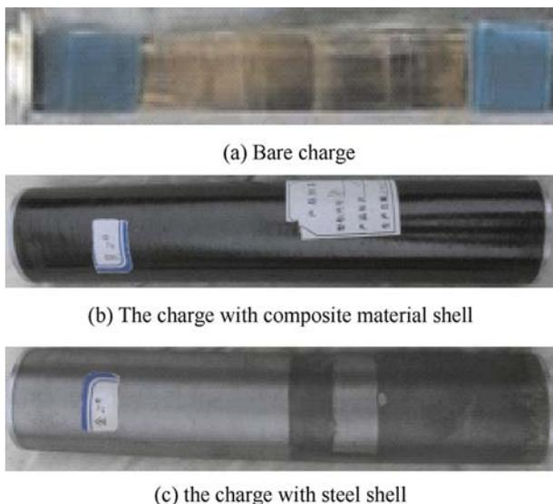
Fig. 1. Schematic diagram of samples.
