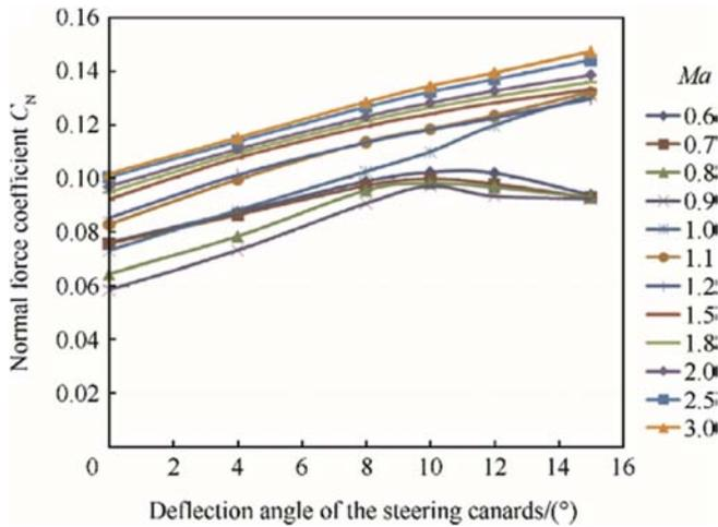
Fig. 8. Changes of the normal force for  $\alpha = 2^\circ$ .
