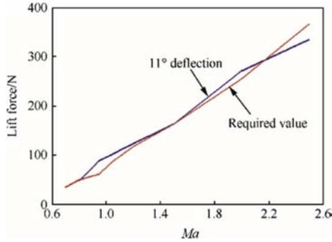
**Fig. 3.** Requirements and capabilities of the steering canards.
