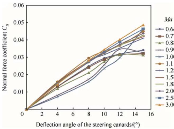
Fig. 7. Changes of the normal force for  $\alpha = 0^\circ$ .
