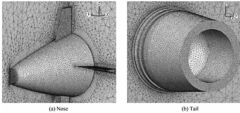
Fig. 6. Meshing at the head and tail of the 2-D guided projectile.
