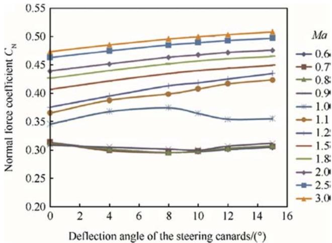
Fig. 11. Changes of the normal force for  $\alpha = 8^\circ$ .
