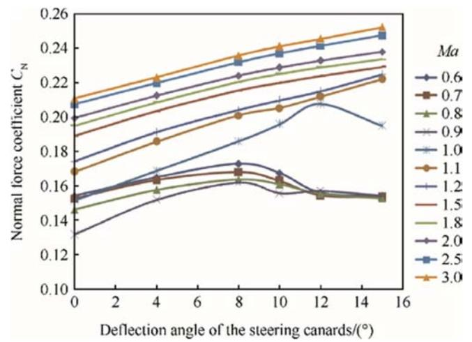
Fig. 9. Changes of the normal force for  $\alpha = 4^\circ$ .
