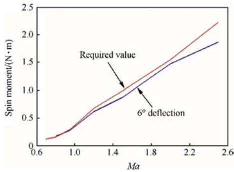
**Fig. 4.** Requirements and capabilities of the spin canards.
