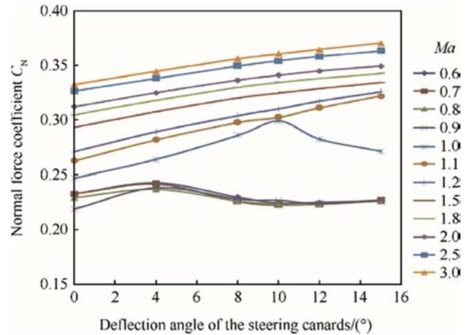
Fig. 10. Changes of the normal force for  $\alpha = 6^\circ$ .
