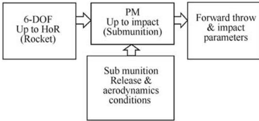
Fig. 2. Flow chart of simulation.
