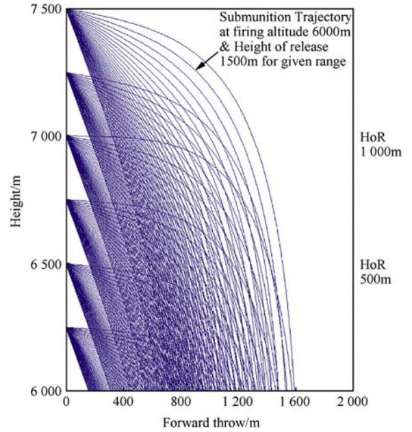
Fig. 10. Trajectory envelope of submunition for different heights and release angles. Altitude = 6000 m from MSL. The trajectory height (Y) of the submunitions at different height of release is plotted in the vertical axis against the distance travel by submunitions (X) or forward throw, in the horizontal axis. It is observed that, the forward throw increases with higher firing altitude as compared to sea level firing for all height of release.
