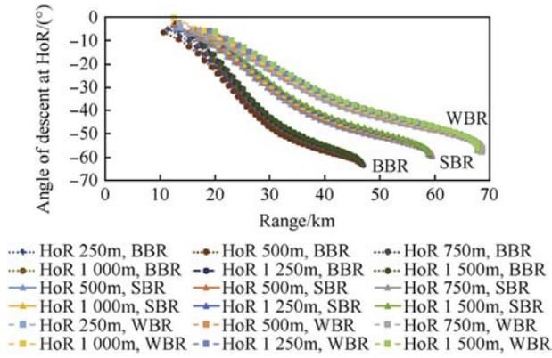
Fig. 8. Release angle vs. range altitude = 6000 m from MSL.
