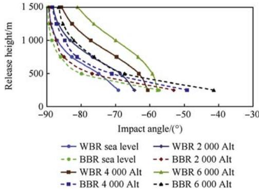
Fig. 12. Release height vs. impact angle.
