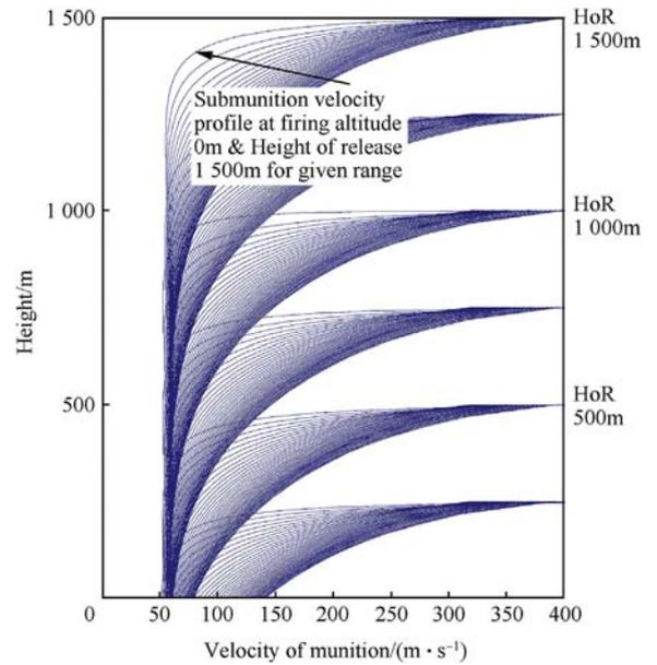
Fig. 11. Velocity vs. release height at various ranges. Altitude = 6000 m from MSL (see Table 2).
