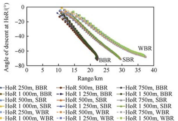
Fig. 7. Release angle vs. range altitude = 0 m from MSL.
