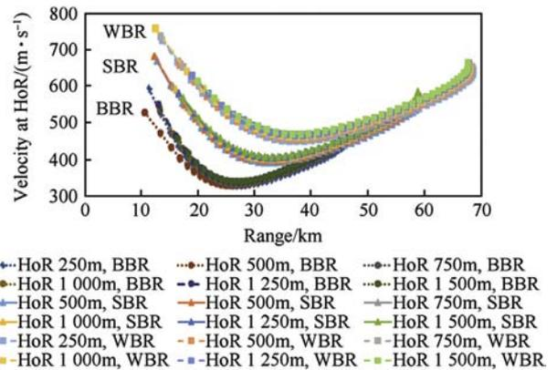
Fig. 6. Release velocity vs. range altitude = 6000 m from MSL. Angle of descent at release height increases with respect to range. For maximum range, it reaches to ~ 70° at sea level and 63° at high altitude conditions as shown in Figs. 7 and 8, for different conditions.
