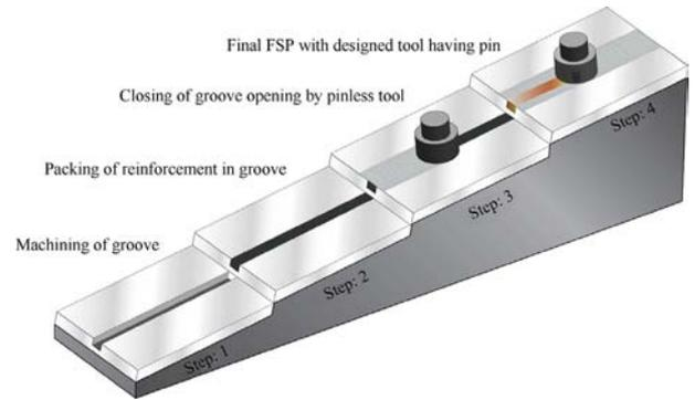
Fig. 2. Steps in SCs fabrication using groove technique.
