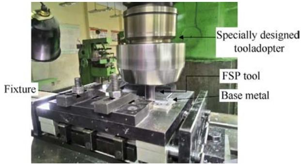
Fig. 3. FSP setup.
