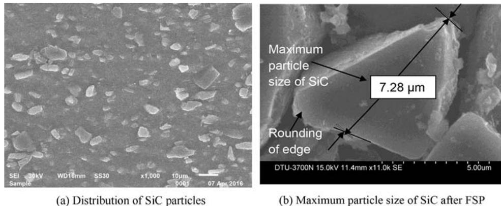
Fig. 5. shows the SEM images of SCs fabricated at 0.25 mm plunge depth, (a) distribution of SiC particles; (b) Maximum size of SiC particle after FSP.
