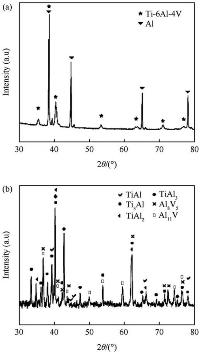
Fig. 5. X-ray diffraction patterns (a) as mixed Ti–6Al–4V powder and Al powder and (b) sample sintered at 1000 °C for 24 h.
