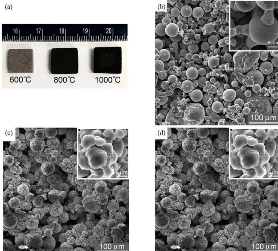
**Fig. 2.** (a) Photograph of sintered samples. SEM micrographs showing surface morphology of samples sintered for 6 h at 600 °C (b), 800 °C (c) and 1000 °C (d). High magnification micrographs are shown in the in-sets.
