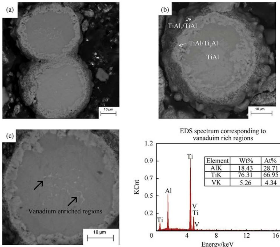
Fig. 4. SEM (BSE) micrograph of the as-polished cross-section of a sample sintered at 1000 °C for 24 h. (a) Region showing the inter-particle bonding region. (b) An individual particle cross-section showing multiple layers.
