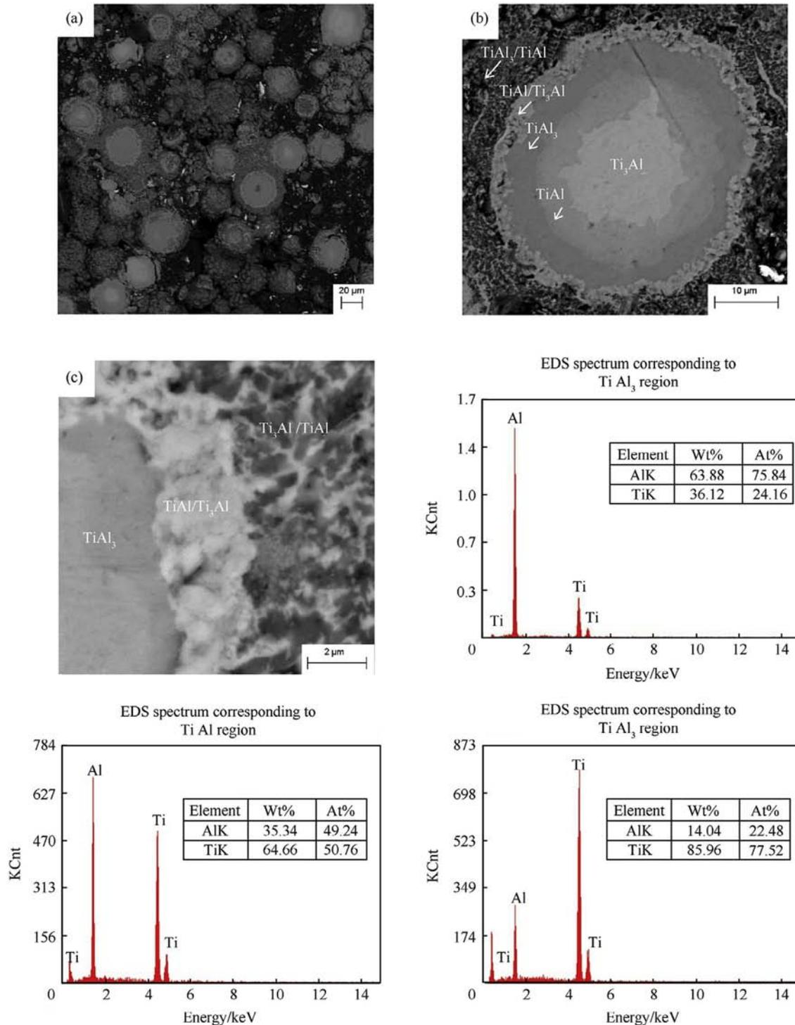
**Fig. 3.** An SEM (BSE) micrograph of the polished cross-section of a sample sintered at 1000 °C for 6 h. (a) Low magnification micrograph showing overall microstructural features. (b) Individual particle cross-section showing different layers of reaction products. (c) High magnification micrograph showing finer features at the first and second layer interface.
